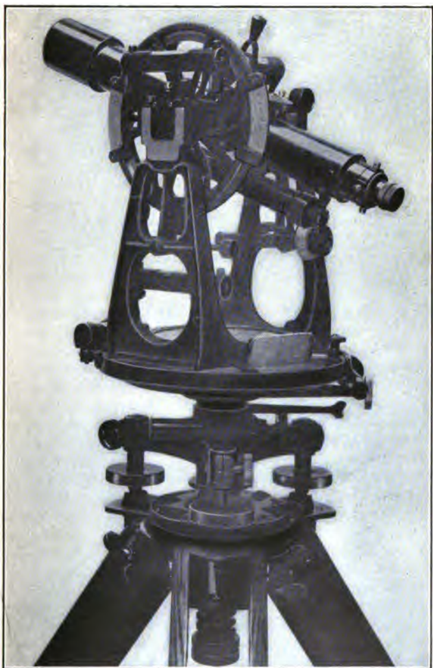
PLATE IV.—ENGINEERS' COMPLETE TRANSIT. (From photograph furnished by C. L. Berger & Sons.) (Facing page 48.)
